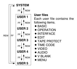
$m{3}$  To enter the selection made in step  $m{2}$  for the user file which is to be used, press the SET button. The user file is changed and stored in the memory.
